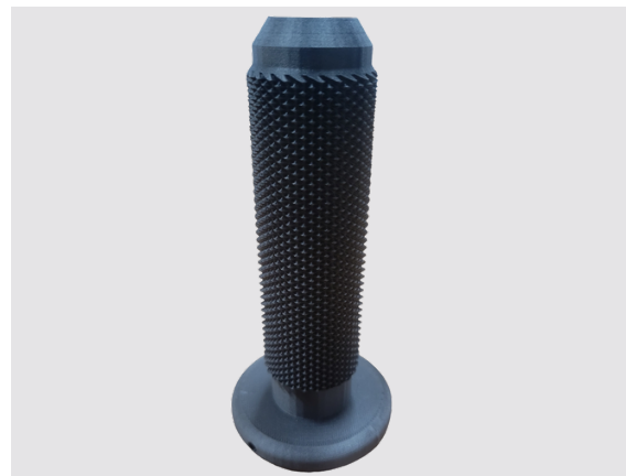
CMarkforged X7 Composite: No set-ups, one material, no CNC finishing.
