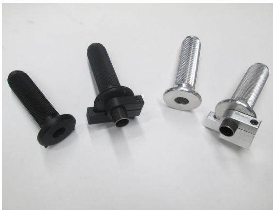
Machined Aluminum: Four total set-ups (two on a CNC Lathe and two on a CNC Mill). Uses two different stocks of raw material.
